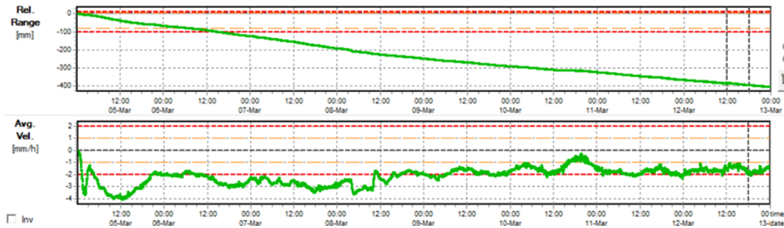
Figure 3. An example of alarm thresholds set that are too ‘tight’, and will result in multiple false alarms.
