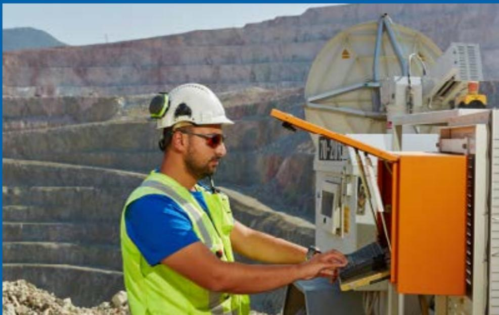
atmospheric conditions since August 2011. Movements can be detected to millimeter accuracy, depending on the range. There are two Movement and Surveying Radars serving in Kışladağ Mine with geo-referenced Geo-camera to get full coverage of the near circular geometry of Kışladağ open pit.
