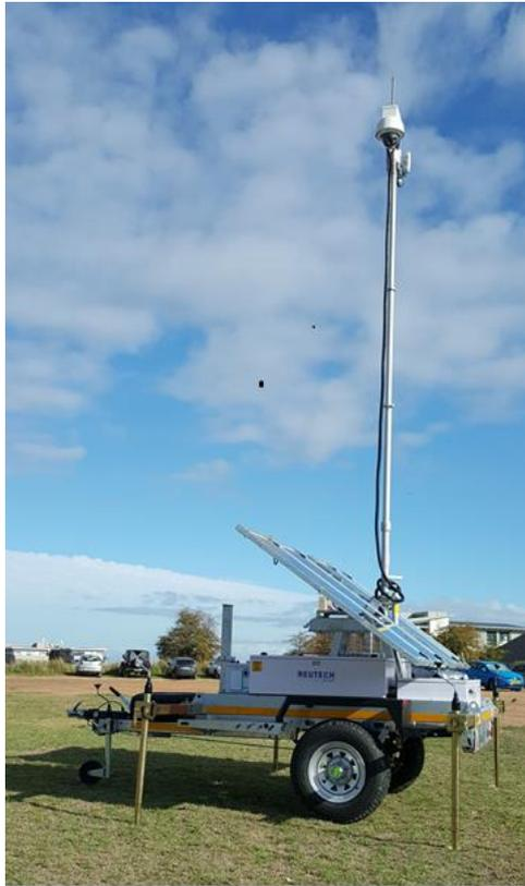
*MPP in WiFi repeater configuration with Slope Vision fitted.*
